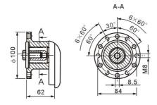
S Splined shaft 1 1/2in 23 T 16/32DP<sup>1)</sup> (SAE J744)
