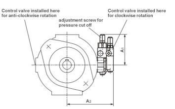
On sizes 28 to 100 the DFR valve used has the flow control spool blocked in the factory and is not tested.  $\label{eq:control}$
