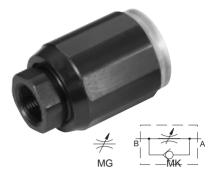
MG/MK series throttle/throttle check valves mounted on the oil pipe lines directly. MG throttle valve is used to regulate flow by turning adjustment sleeve. MK throttle check valve is used to control flow in one direction and allow free flow in the opposite.
