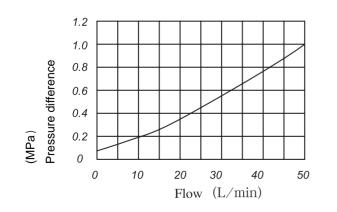
Z4S16 Rectifier sandwich place curves Flow direction from A to B (B to A)
